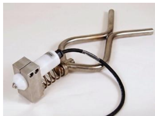
CP probe mounted in Springy Fishtail handle
