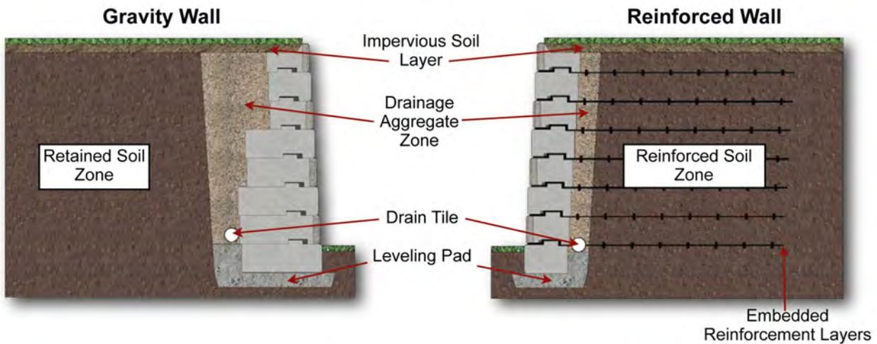
The soils that are of critical interest to a wall designer are categorized into five basic zones with respect to their location in and around the finished wall.
