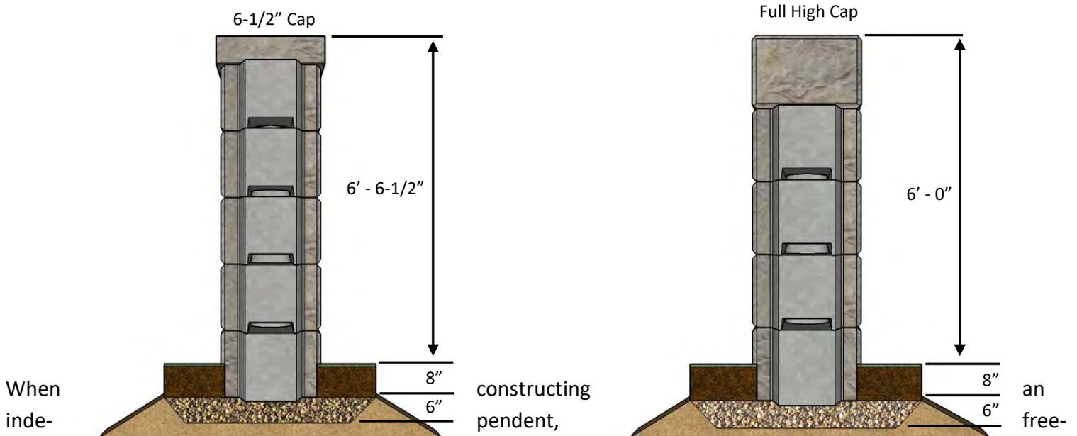
standing wall it is important that the foundation soils be properly prepared and compacted to provide adequate support for the wall. When freestanding blocks are installed in combination with a retaining wall (as the top of wall finish), the wall and foundation soils should be analyzed for the addition of the freestanding block weight.
