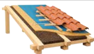
PITCHED ROOF WITH INTERNAL ISULATION BETWEEN RAFTERS
