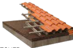
PITCHED ROOF WITH RIGID INSULATION OVER SLAB
