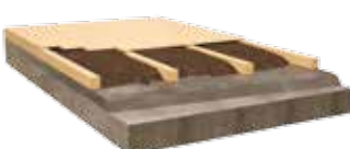
BETWEEN JOISTS LOOSE FILL
