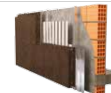
EXTERIOR CLADDING WITH SHIPLAP SYSTEM - CORK AT SIGHT
