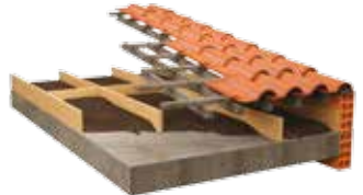
PITCHED ROOF WITH LOOSE FILL INSULATION BETWEEN JOISTS
