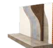
INTERNAL INSULATION FOR EXTERNAL WALLS
