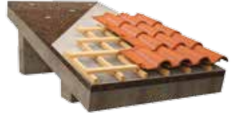
PITCHED ROOF WITH ROOF MEMBRANE
