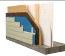
STANDARD LAP SIDING WITH EXTERIOR RIGID INSULATION
