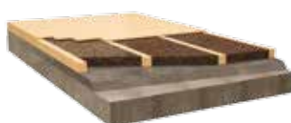
FLOORING JOISTS CAVITY FILLING
