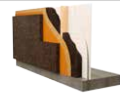
EXTERIOR CLADDING OVER WOODEN SUBSTRATE - CORK AT SIGHT
