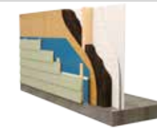
STANDARD LAP SIDING WITH CAVITY INSULATION
