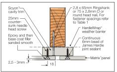
FIGURE 21 COUNTERSUNK SCREW OPTION 3
