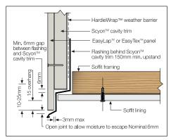
FIGURE 33 FACADE/SOFFIT JUNCTION
