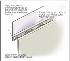
FIGURE 11 JOINT SEALANT OPTION 1
