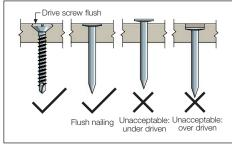
FIGURE 2 NAIL FASTENER DEPTH
