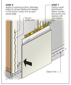
FIGURE 14 INSTALL FIRST PANEL
