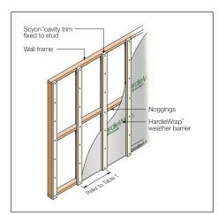
FIGURE 4 ON-STUD FIXING
