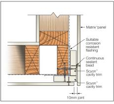
FIGURE 28 EXTERNAL CORNER DETAIL
