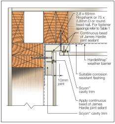
FIGURE 29 INTERNAL CORNER DETAIL
