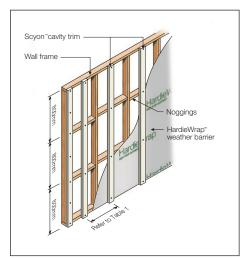
FIGURE 5 OFF-STUD FIXING
