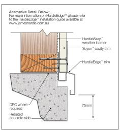
FIGURE 9B ALTERNATIVE SLAB EDGE DETAIL
