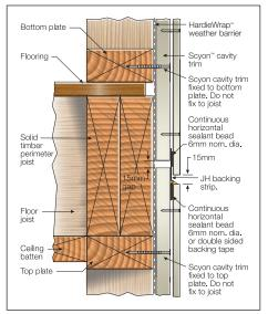
FIGURE 30 FLOOR LEVEL JUNCTION
