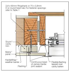
FIGURE 25 WINDOW JAMB DETAIL
