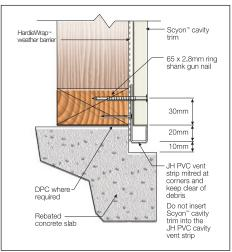
FIGURE 9A SLAB EDGE DETAIL
