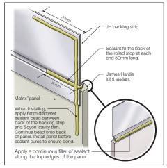
FIGURE 13 SEALING JH BACKING STRIP END DETAIL
