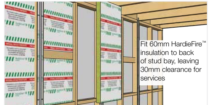
FIGURE 20 HARDIEFIRE™ INSTALLATION
