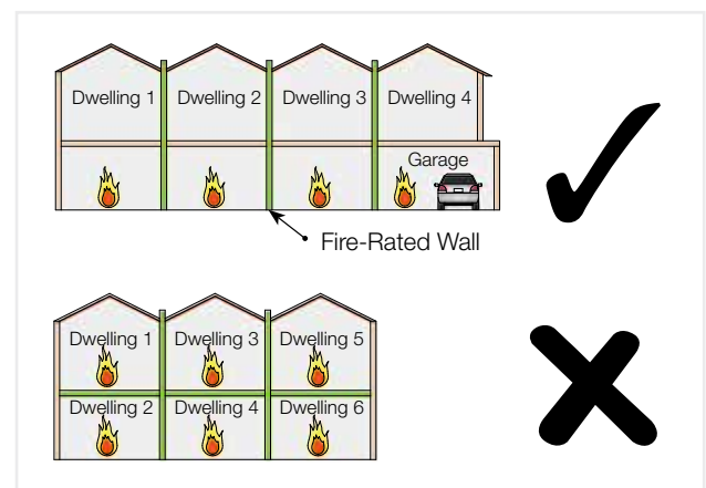
FIGURE 1 HARDIESMART™ INTERTENANCY WALL SYSTEM TYPICAL APPLICATIONS
