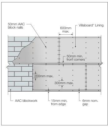
FIGURE 14 AAC - HORIZONTAL LAYOUT
