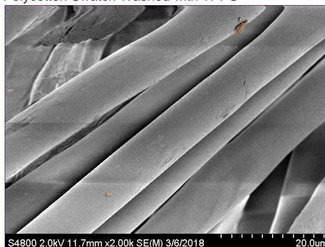
Figure 2. SEM Scan of Polyester Fibers on Polycotton Swatch Washed with TPFG
