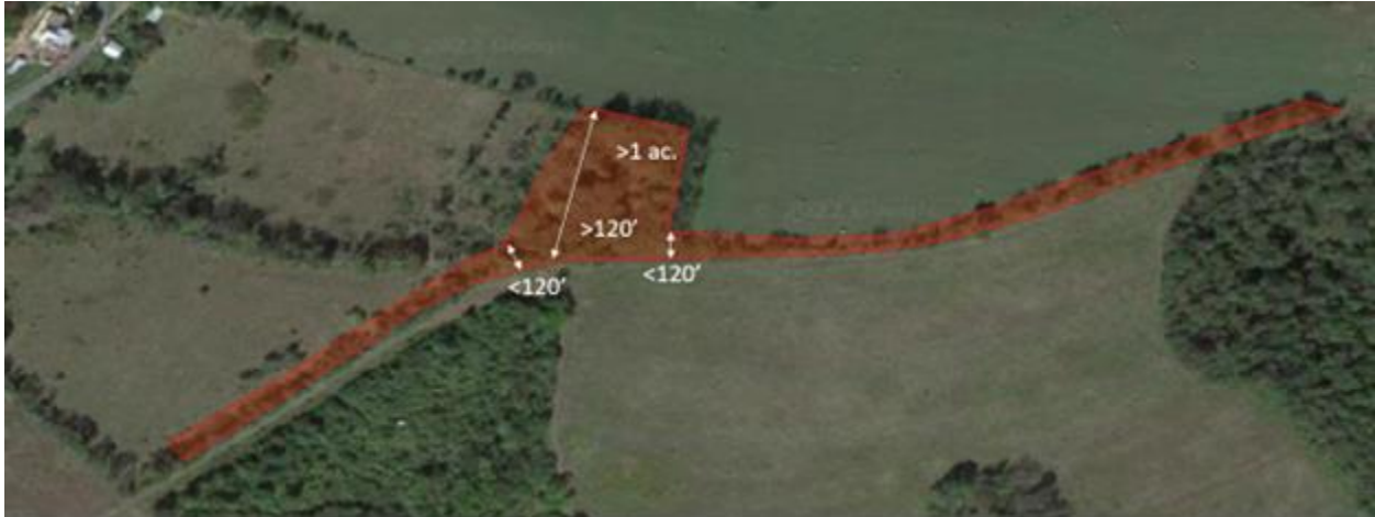
Figure 1. The area in question (red) is greater than 1 acre, but it includes areas with tree cover that are less than 120' wide. However, at its widest, the area is at least 120' wide, so the entire polygon is included.
