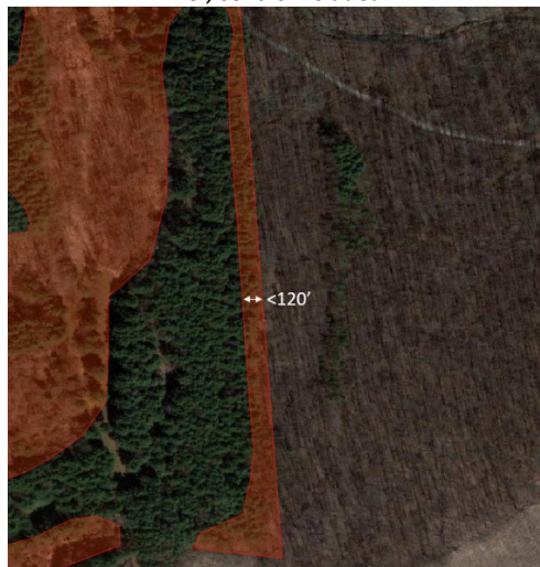
Figure 3. Even though the area in question (red) is less than 120' wide, it is a component of a larger forested block that is at least one acre in area and at least 120' wide. Thus, the area is included.
