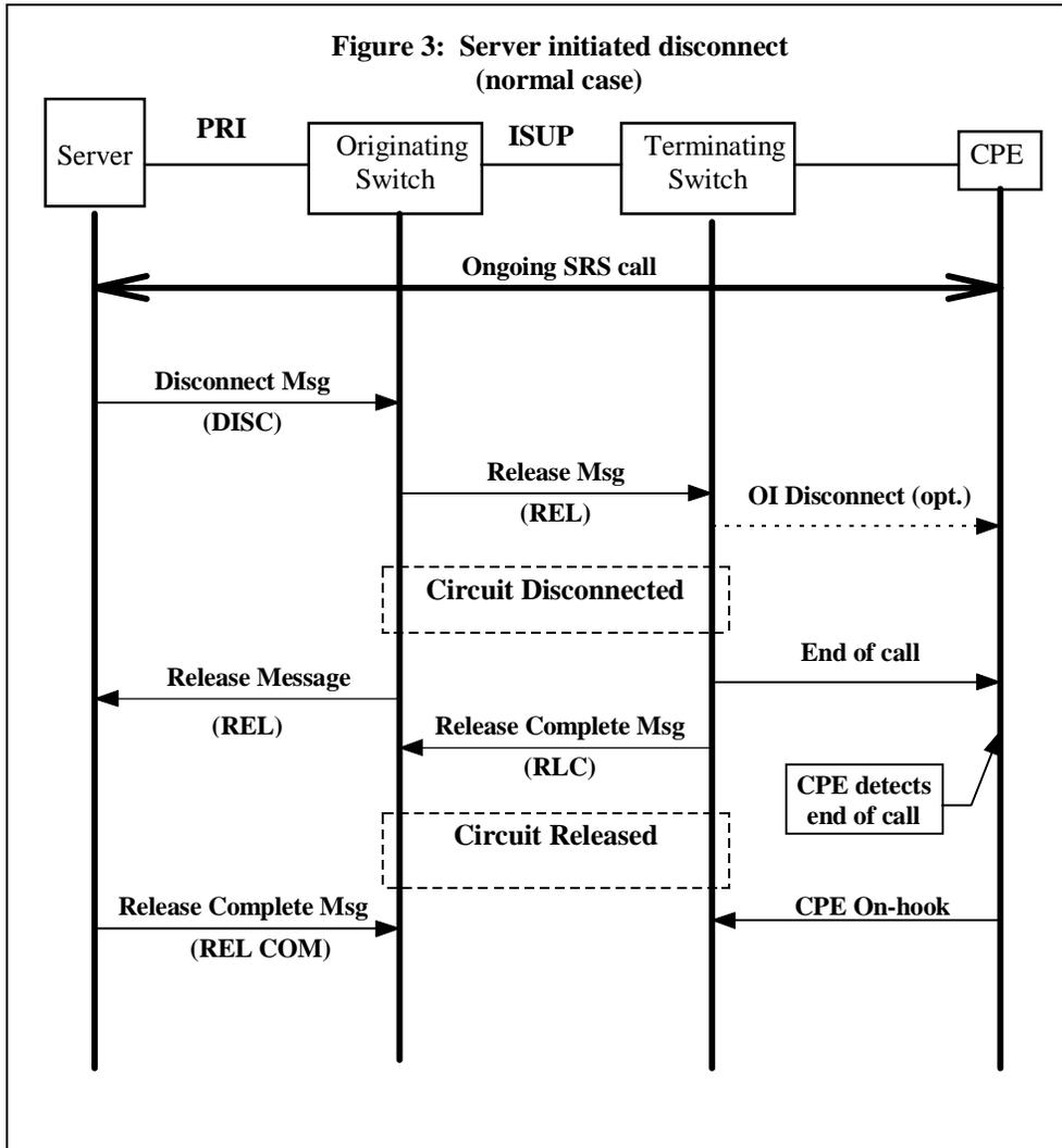
A suppressed ringing call will normally be disconnected by the server after the data transmission is completed. Figure 3 shows this call disconnect message flow.
