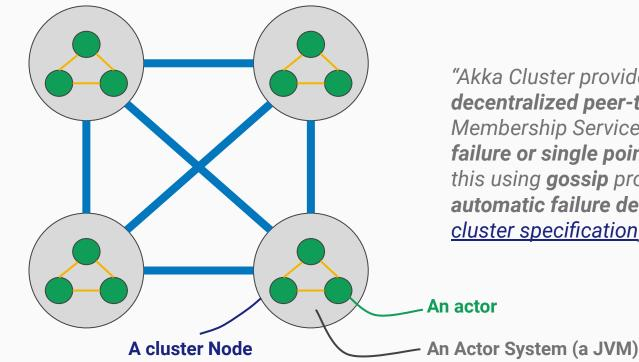
"Akka Cluster provides a **fault-tolerant decentralized peer-to-peer** based Cluster Membership Service with **no single point of failure or single point of bottleneck**. It does this using **gossip** protocols and an **automatic failure detector.**" (<u>Akka doc -</u> <u>cluster specification</u>)
