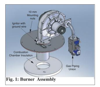
Remove the Phillips head screws attaching the burner head to the burner mounting plate. Inspect the burner head for deterioration. Replace if necessary.
