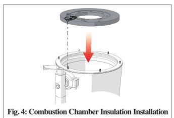
19. Check combustion chamber insulation alignment with the burner mounting plate. The combustion chamber insulation igniter cutout should align with the opening in the burner mounting plate. If not properly aligned, remove the burner mounting plate and reposition combustion chamber insulation.
