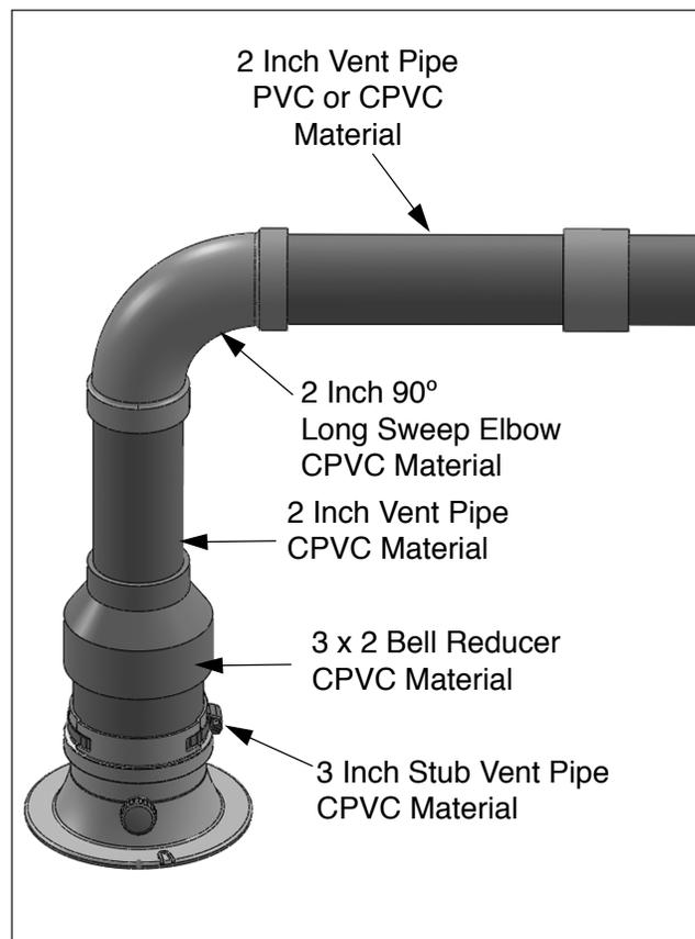
Fig. 21 - 2" CPVC/PVC Venting System Horizontal
