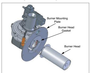
Fig. 2: Burner Head and Gasket Assembly
