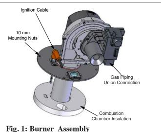
6. Remove the 10 mm mounting nuts and remove the burner assembly from the HEAT EXCHANGER body.
