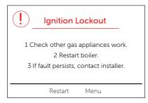
To restart the boiler, press Restart. The boiler will repeat the ignition sequence. If the boiler still fails to light consult a Registered Gas Installer.
