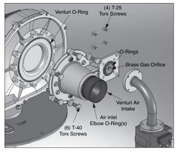
Fig. 2: Venturi/Gas Orifice Assembly
