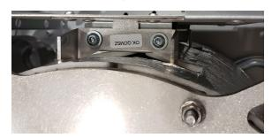
Fig. 11: Heat Exchanger Bracket Screws
