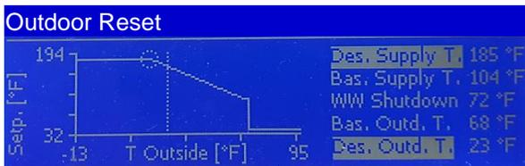
It's now possible to set the Outdoor reset curve by changing the parameters on the righthand of the screen.
