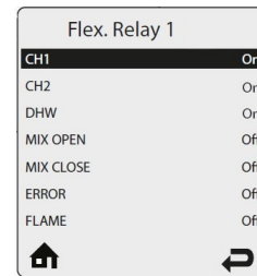
Fig. 15: Flex. Relay 1 Settings
