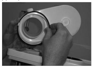
2. Place the New Adaptor onto the top of the Challenger, positioning the flue tube inside the adaptor. The test port should face the front of the Challenger and the o-ring should fit into the top cover of the Challenger.
