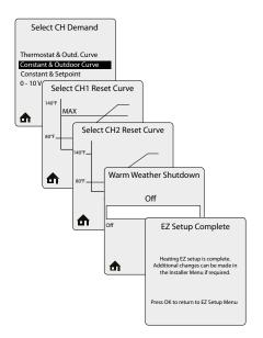
**Constant & Outdoor Curve -** The EXALT will maintain setpoint without an external CH call from a thermostat or zone panel. The setpoint will vary with the outdoor temperature for central heating calls. After Constant & Outdoor Curve is selected, the **Select CH1 Reset Curve** screen appears
