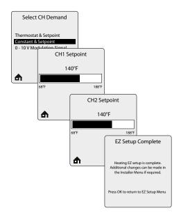
**Constant & Setpoint** - The EXALT will maintain setpoint without an external CH call from a thermostat or zone panel. The setpoint will be fixed for CH calls. After Constant & Setpoint is selected, the CH1 Setpoint screen appears.
