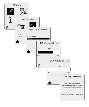
When **Sensor** is selected in Select DHW Demand, use of an (optional) Indirect Water Heater Sensor is required. The EXALT monitors the DHW storage temperature and generates a DHW call whenever the temperature drops below the DHW storage setpoint by 6°F [3°C].
