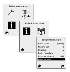
**Boiler Information** provides real time operating information of the EXALT. Each line contains an information item followed by its current value. Six lines are displayed on the screen at one time.
