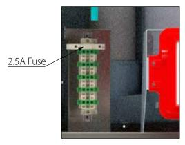
Fig. 25 - Terminal Strip Location
