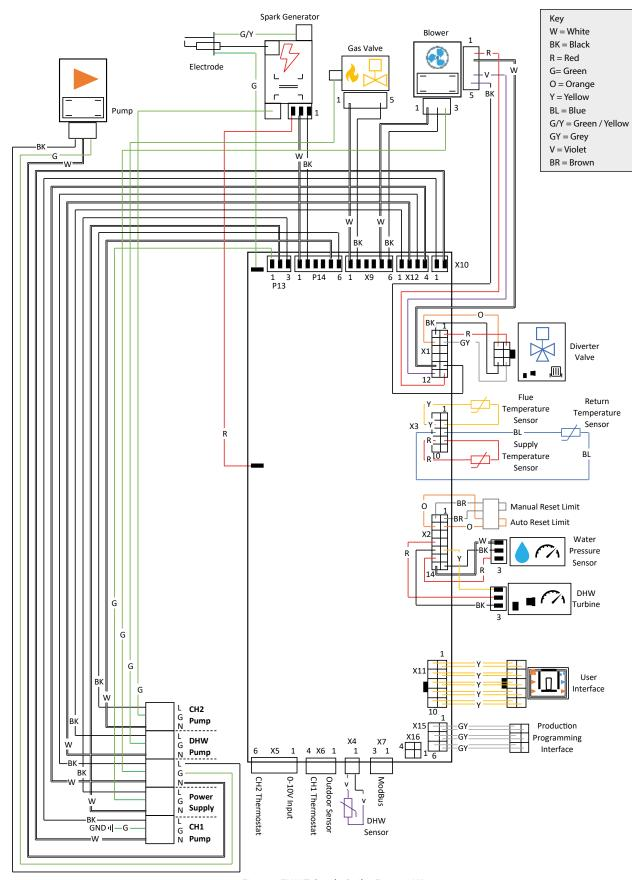
Fig. 23 - EXALT Combi Boiler Factory Wiring
