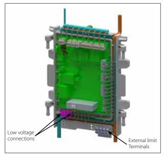
Fig. 26 - Low Voltage Connections
