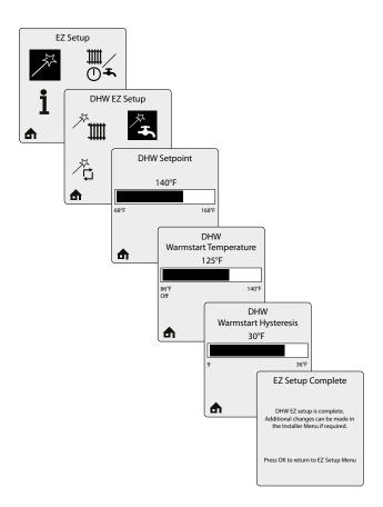
**DHW EZ Setup** prompts the installer to select the DHW setpoint.
