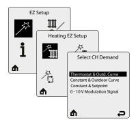
**Select CH Demand** prompts the installer to select how a CH Demand is generated. **Thermostat & Outd. Curve** – A central heating call from a thermostat or zone panel w
