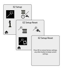
EZ Setup Reset allows reset of all EZ Setup settings back to the original factory defaults. See**Chapter 13** for the list of settings reset by this function.
