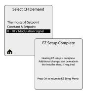
**0 - 10V Modulation Signal** - This option allows the EXALT firing rate to be controlled by an external control system.
