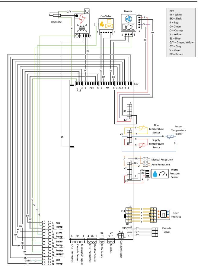
Fig. 22 - EXALT Heat Only Boiler Factory Wiring
