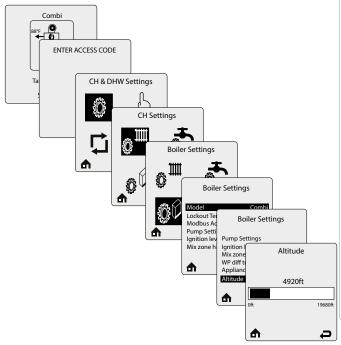
**Altitude** must be correctly set to allow reliable operation of the boiler.
