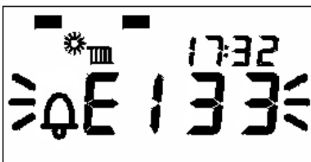
Fig 7.3.3 - Boiler Display With Low Inlet Gas Pressure
