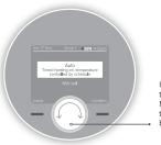
Use the dial to scroll between the different modes (Auto, Manual and Off) and then push the dial or press the right hand button to confirm your selection
