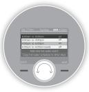
Push the dial to edit a hot water time or temperature when it is highlighted in light blue. You can also add an additional heating period by scrolling and pushing on the "Add new hot water event" bar. You can have up to 6 hot water events per day in your schedule.
