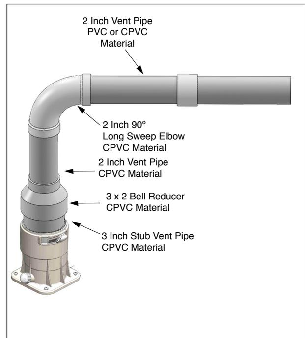
Fig. 22 - 2" (60 mm) CPVC/PVC Venting System Horizontal
