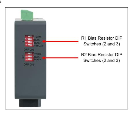
To enable Bias Resistors, move the BIAS- and BIAS+ DIP switches to the right in the orientation shown above.
