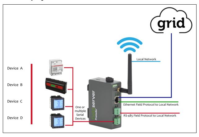
The ProtoAir can connect with the MSA Grid – FieldServer Manager. The FieldServer Manager allows technicians, the OEM's support team and MSA Safety's support team to remotely connect to the ProtoAir. The FieldServer Manager provides the following capabilities for any registered devices in the field:
