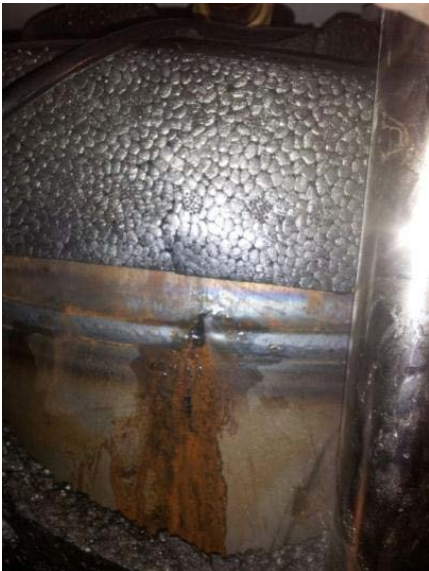
Picture showing failure mode (leak at weld)
