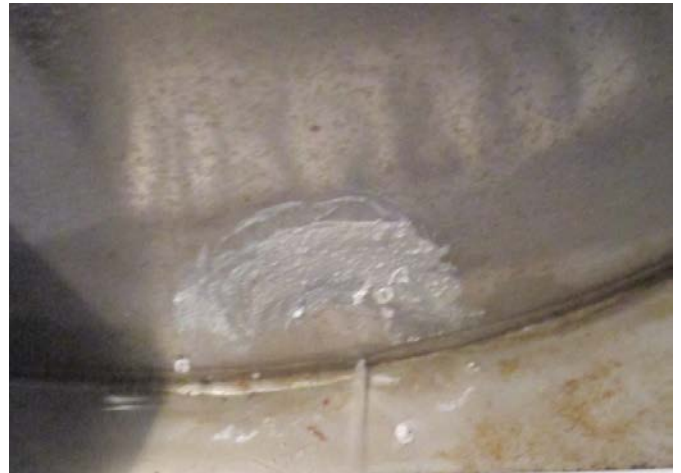
Picture showing failure mode (circular weld leak)
