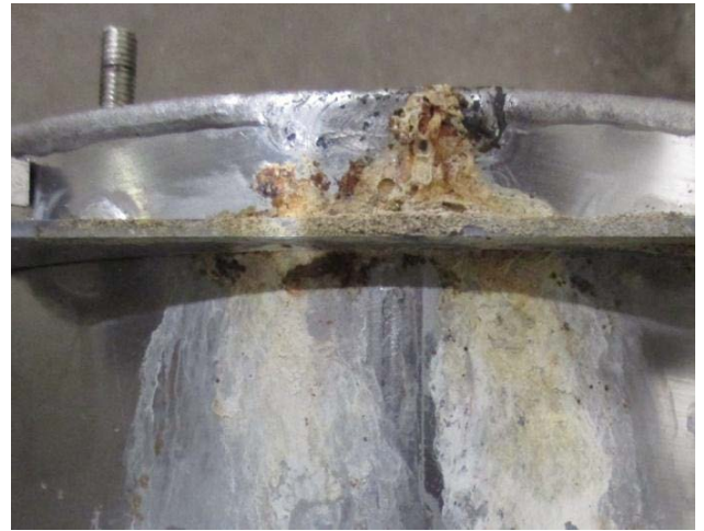
Picture showing failure mode (circular weld leak)
