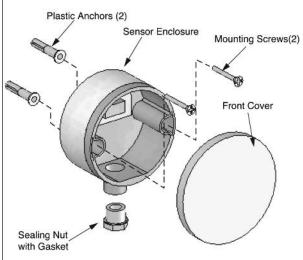
Fig. 25: Sensor Enclosure and Components
