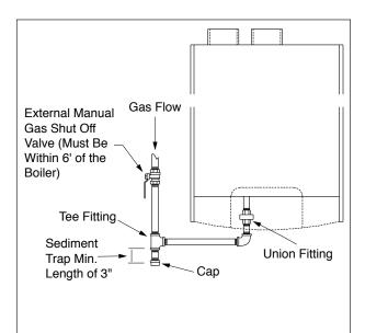
Fig. 16: Recommended Gas Supply Piping
