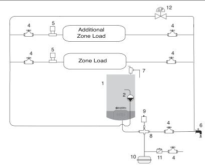
**Note:** Verify CH circulator is properly sized to overcome the system pressure drop and provide adequate flow through the boiler system.
