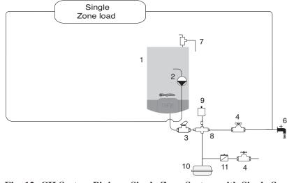
**Note:** Verify CH circulator is properly sized to overcome the system pressure drop and provide adequate flow through the boiler system.
