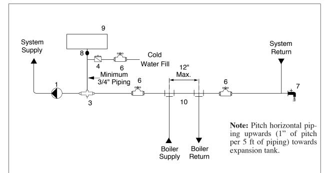
Fig. 7: Near Boiler Piping - Closed Type Expansion Tank
