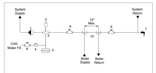
Fig. 6: Near Boiler Piping - Diaphragm Expansion Tank
