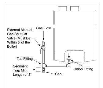
Fig. 16: Recommended Gas Supply Piping
