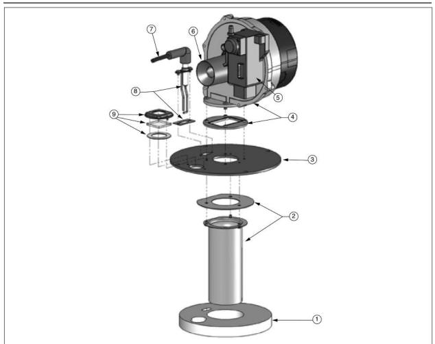
Fig. 28: PRESTIGE Excellence Burner Components
