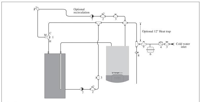
Fig. 6: Domestic Piping with Optional Storage Tank
