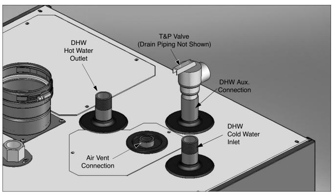
Fig. 2: Standard Installation of the T&P Relief Valve
