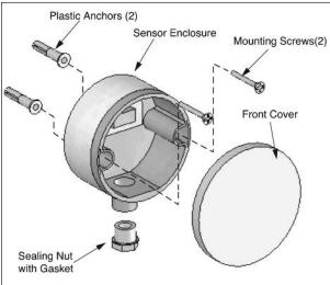
Fig. 25: Sensor Enclosure and Components
