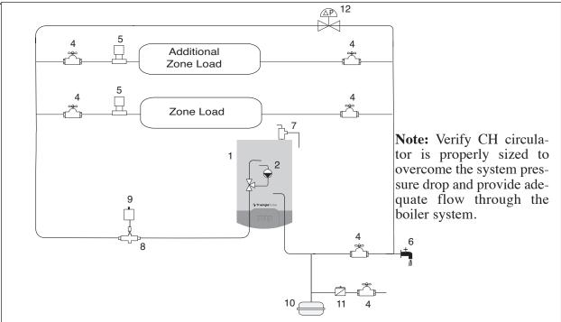
Fig. 11: CH System Piping - Multiple Zone Valve with Single System/Boiler Circulator
