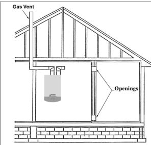
Fig. 1: All Combustion Air from Adjacent **Indoor Spaces Through Indoor Combustion Openings**
