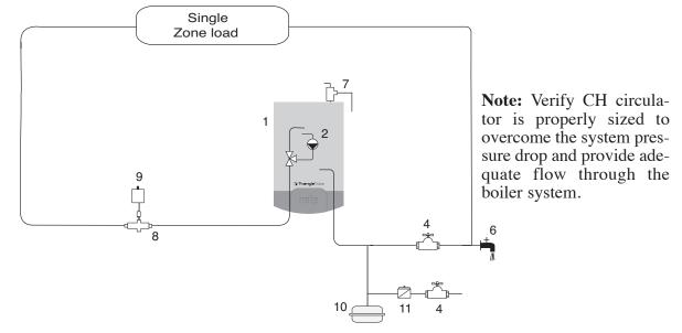
Fig. 12: CH System Piping - Single Zone System with Single System/Boiler Circulator
