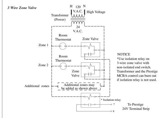
Fig. 22: Multiple Zone Field Wiring Using Zone Valves
