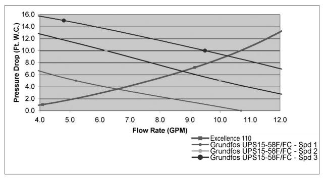
Note: Minimum allowable flow rate at full input: 5.0 gpm
