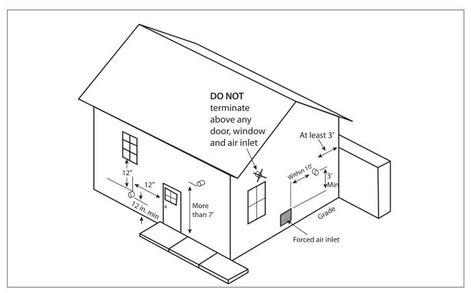
Fig. 2 - Termination Clearances of Direct Vent System
