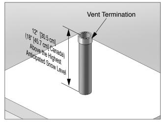
Fig. 15 - Category - IV - Vertical Termination of Vent Pipe
