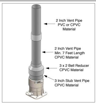
Fig. 21 - 2" (60 mm) CPVC/PVC Venting System Vertical
