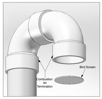
Fig. 3 - Vertical Vent Bird Screen Installation
