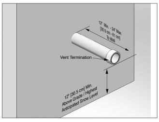
Fig. 18 - Category IV - Sidewall Termination of Vent Pipe
