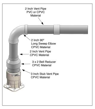
Fig. 22 - 2" (60 mm) CPVC/PVC Venting System Horizontal
