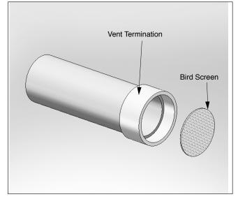
Fig. 9 - Sidewall Vent Bird Screen Installation
