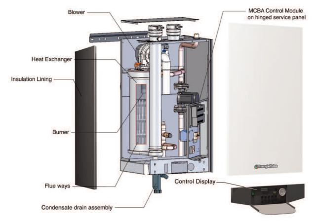
The components of the Prestige are easily accessible for serviceability. The Solo 60,175, 250 & 399 are shipped less the circulator.
