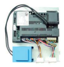
The Prestige uses a microprocessor electronic control module that automatically adjusts blower speed and gas flow rate to modulate boiler firing rate to closely match boiler output to space heating or DHW heating demand. The module responds to signals from the room thermostat, supply and return water temperature sensors, flue temperature sensor, domestic hot water aquastat and outdoor temperature sensor.
