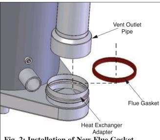
Fig. 2: Installation of New Flue Gasket
