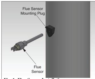
Fig. 1: Flue Sensor Installation
