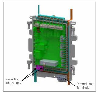
Fig. 26 - Low Voltage Connections
