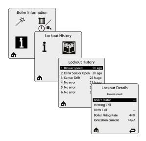
**Lockout History** records the last eight lockouts. Six lines are displayed on the Lockout History screen at one time. Each line contains a lockout description followed by how long ago the lockout occurred.
