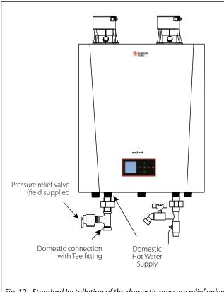
Fig. 12 - Standard Installation of the domestic pressure relief valve
