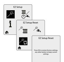
EZ Setup Reset allows reset of all EZ Setup settings back to the original factory defaults. See**Chapter 13** for the list of settings reset by this function.
