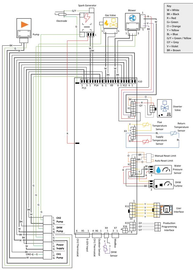
Fig. 23 - INSTINCT Combi Boiler Factory Wiring
