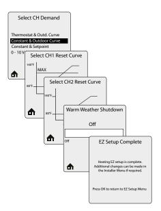
**Constant & Outdoor Curve -** The INSTINCT will maintain setpoint without an external CH call from a thermostat or zone panel. The setpoint will vary with the outdoor temperature for central heating calls. After Constant & Outdoor Curve is selected, the **Select CH1 Reset Curve** screen appears
