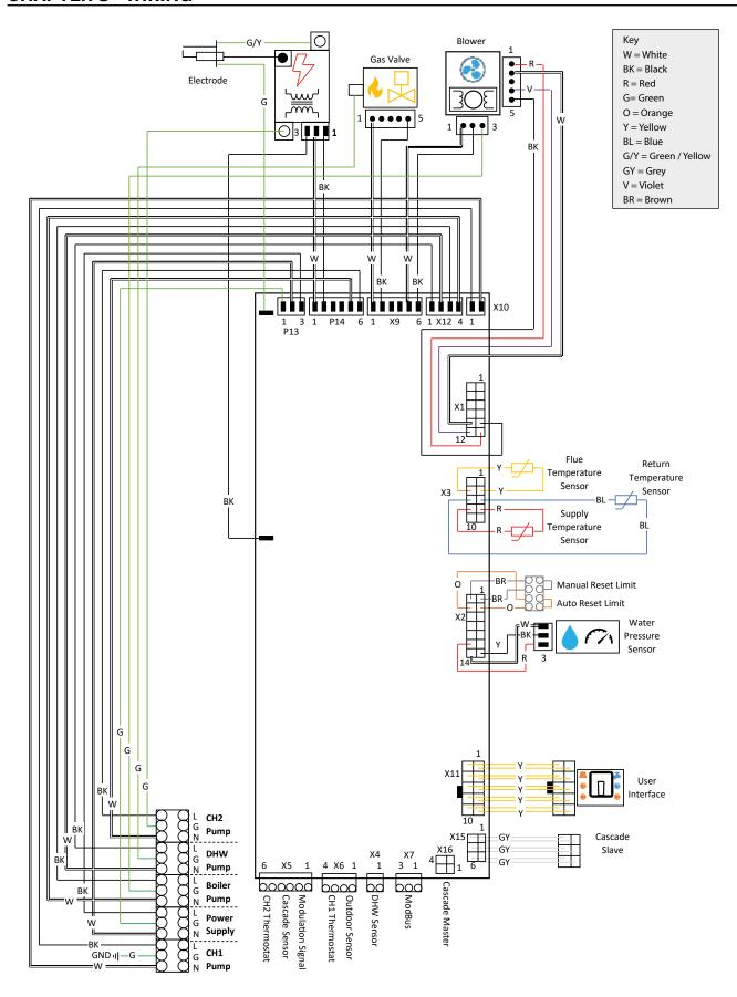
Fig. 22 - INSTINCT Solo Boiler Factory Wiring
