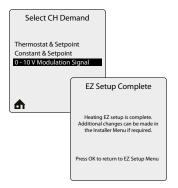
**0 - 10V Modulation Signal** - This option allows the INSTINCT firing rate to be controlled by an external control system.
