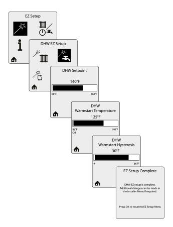
**DHW EZ Setup** prompts the installer to select the DHW setpoint.
