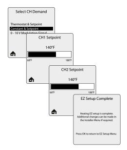
**Constant & Setpoint** - The INSTINCT will maintain setpoint without an external CH call from a thermostat or zone panel. The setpoint will be fixed for CH calls. After Constant & Setpoint is selected, the CH1 Setpoint screen appears.
