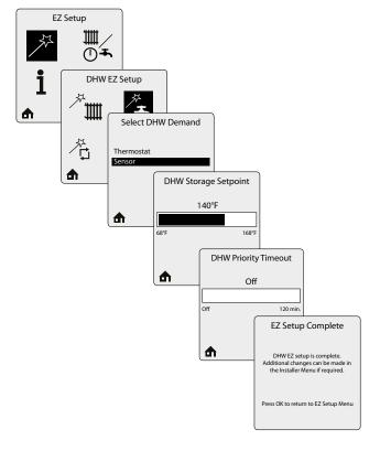
When **Sensor** is selected in Select DHW Demand, use of an (optional) Indirect Water Heater Sensor is required. The INSTINCT monitors the DHW storage temperature and generates a DHW call whenever the temperature drops below the DHW storage setpoint by 6°F [3°C].
