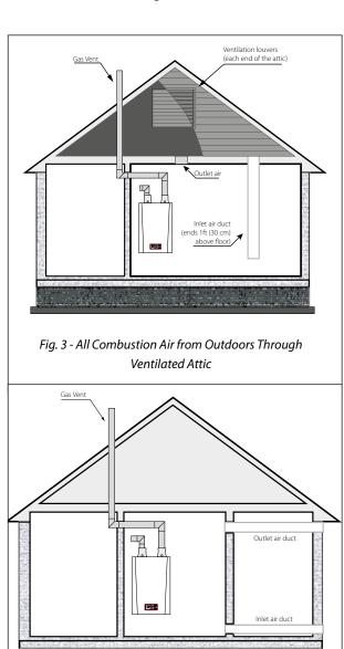
Fig. 4 - All Combustion Air from Outdoors Through
