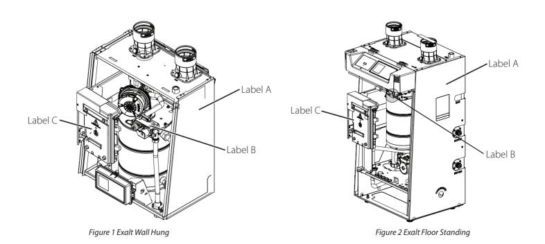
The Propane Rating Label (D) must be placed on top of the boiler performance data of the original rating label, leaving the top section of the original rating plate exposed.
