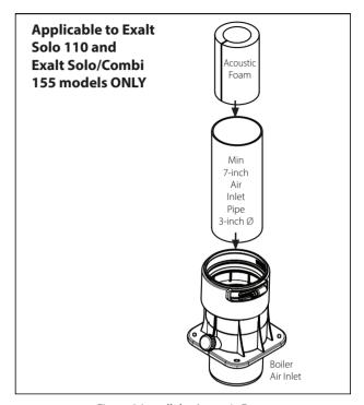
Figure 3 Install the Acoustic Foam
