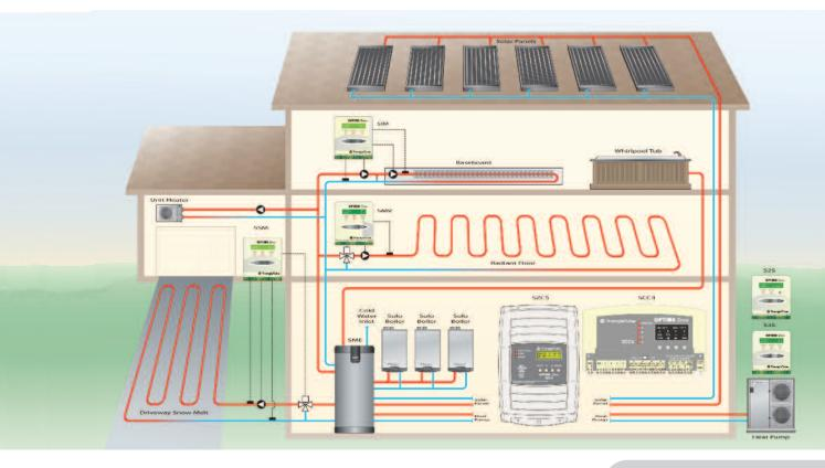
Triangle Tube's Optima Series Hydronic Controls are designed to optimize the performance of hydronic heating and domestic hot water systems. Optima Series boiler controls effectively manage multiple heat sources to maintain the desired comfort level. The Optima Series sytem controls can manage multiple zones and temperatures within the system.
