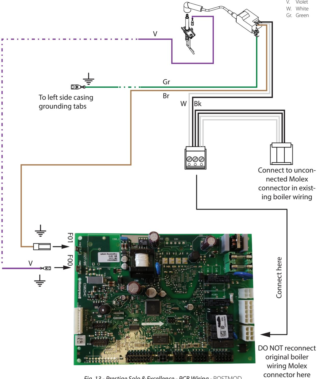
Fig. 13 - Prestige Solo & Excellence - PCB Wiring - POSTMOD
