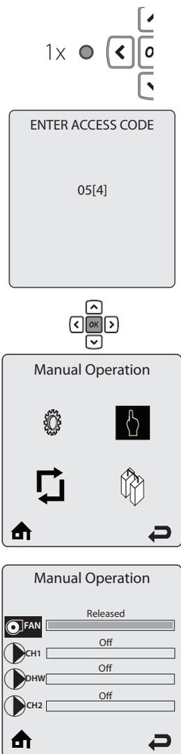
Fig. 9 - Accessing the Combustion Adjustment Interface
