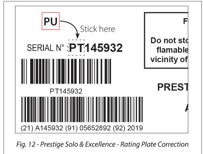
Fig. 12 - Prestige Solo & Excellence - Rating Plate Correction
