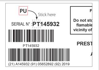
Fig. 12 - Prestige Solo & Excellence - Rating Plate Correction
