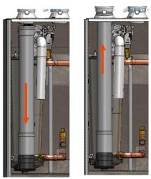
Fig. 8 - - Venting pipe with telescopic section
