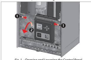
Fig. 1 - Opening and Lowering the Control Panel
