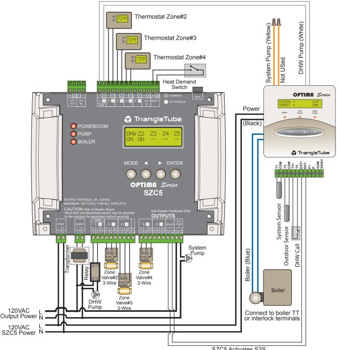
SZC5 Activates S3S Connect SZC5 Boiler Output to S3S EXT± Enable/Disable Input
