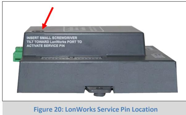
Figure 20: LonWorks Service Pin Location
