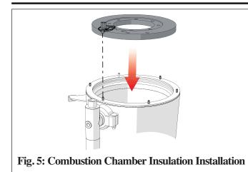
20. Check combustion chamber insulation alignment with the burner mounting plate. The combustion chamber insulation igniter cutout should align with the opening in the burner mounting plate. If not properly aligned, remove the burner mounting plate and reposition combustion chamber insulation.
