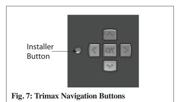
2. Enter the installer access code "054" by using the LEFT and RIGHT buttons to select a digit and the UP and DOWN buttons to change the digit. Press the OK button to enter the access code.
