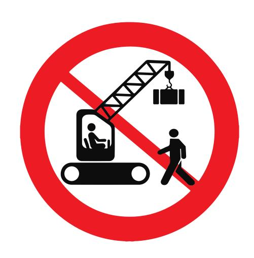
**07.** Follow the lift plan and do not walk under a suspended load.
