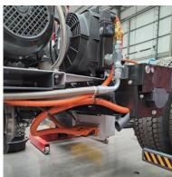
6. Cut ties along the short loom up to the charge socket and let the cable hang
