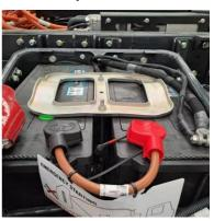
2. Locate + Remove both Master Service Disconnect devices (MSD) – see
