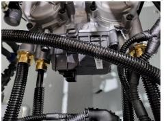
3. Remove the 5x air pipes, 4x on top and 1x underneath, using an air pipe removal tool and pushing against the collar whilst pushing in the air pipes before pulling out, making sure to note the location of each pipes fitment
