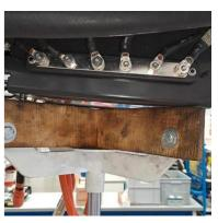
16. Unfasten and remove the two bolts securing the earth bus bar and place bus bar onto a clean secure workstation
