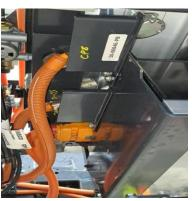
7. Remove the HV cable from the side of the KEB (unfasten Torx 20 Bolts)
