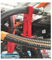
11. Clamp off and disconnect the two DC/DC coolant hoses via the release tags on the connections.
