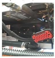
9. Release the cable clip from the BMS housing and temporarily adjust location of loom to the side of the KEB
