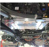
6. Unfasten the two HV security brackets and disconnect the KEB
