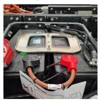
Locate + Remove both Master Service Disconnect devices (MSD) – see Master Service Disconnect Remove/Refit
