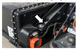
9. Lower hydraulic lift and battery assembly from vehicle
