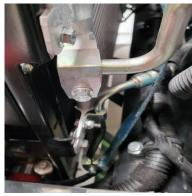
14. Remove the 2x 15 mm radiator side mounting bolts (note: it may be necessary to cut some of the cable ties securing the hoses on the n/s to gain access to the n/s bolt
