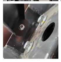
10. Remove radiator cooling fan by first disconnecting the multiplug & undoing 8x 10 mm nuts, then using a suitable trim tool, slowly prise the fan off of the studs
