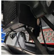
12. Attach a suitable strap to support the air con condenser (being very careful not to damage the fins), so it can be removed from the radiator but without having to disconnect and de-gas the air conditioning
