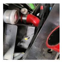
16. Remove lower o/s radiator hose by undoing the 10 mm jubilee clip
