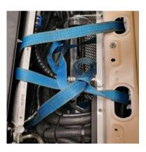
13. Remove the condenser by undoing the 4x 10 mm nuts and bolts, two either side of the condenser, gently move aside
