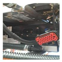
9. Release the cable clip from the BMS housing and move loom to the side
