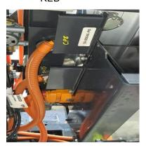
7. Remove the HV cable into the side of the KEB (undo the torx screw T20)
