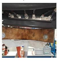
16. Undo and remove the two bolts securing the earth bus bar and place bus bar out the way
