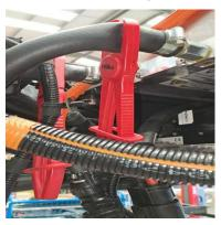
11. Clamp off and disconnect the two DC/DC coolant hoses via the release tags on the connections. Be prepared to catch residual coolant
