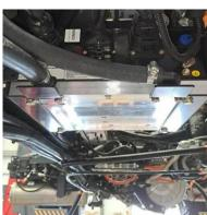
Undo and remove the two HV security brackets and disconnect the KEB
