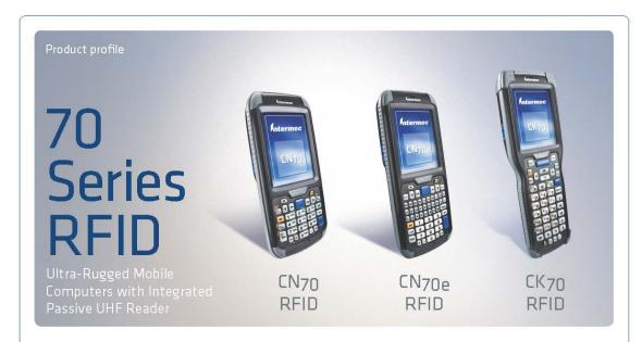
The Intermec 70 Series R FID is the no compromise, next generation family of ultra-rugged mobile computers that combine passive UHF reading with purpose-built designs in one common platform.
