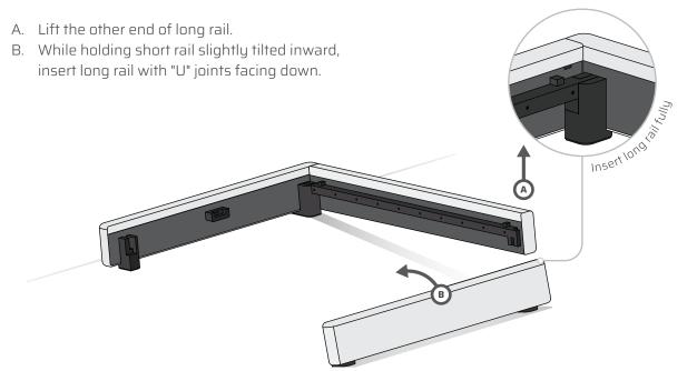
Place the remaining long rail into short rails with the "U" joints facing down. Press it down fully.
